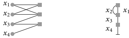
Figure 2.17: Left: A standard FG in which each variable node has degree at most two. Right: The equivalent FSFG. The variables in the FSFG are associated with the edges in the FG.
