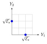
The noise  $Z_1, Z_2 \sim \mathcal{N}\left(0, \frac{N_0}{2}\right)$  and  $Z_1$  is independent of  $Z_2$ . The probability of error can be readily calculated as
