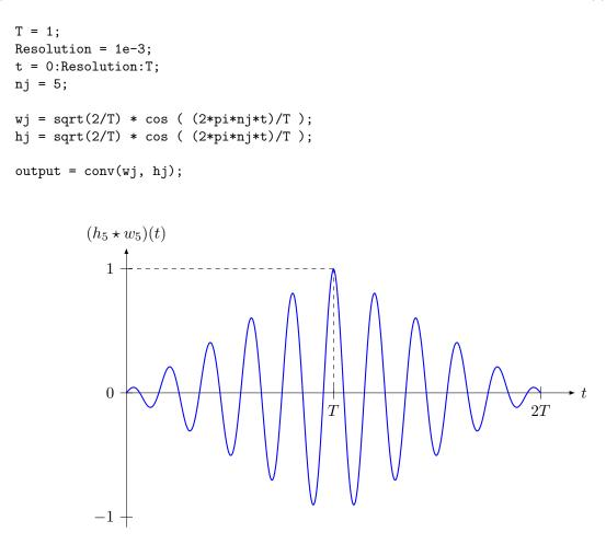
Note that the resulting signal is zero for  $t \leq 0$  and also for  $t \geq 2T$ . The figure also reveals why sampling at time t = T is a good idea: the value of the matched filter output signal is maximal.
