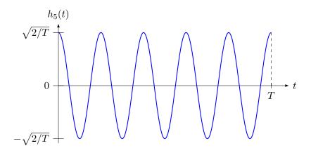
The receiver then processes the received signal R(t) through the matched filter  $h_j(t)$  to obtain  $(R \star h_j)(t)$ . This signal is sampled at time T to yield the value needed for the MAP decision.
