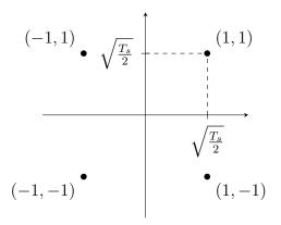
The mapping is such that neighboring points differ by one bit. This minimizes the biterror probability since when we make an error chances are that we choose a neighbor of the correct symbol. Notice that we may decode each bit independently. In fact the first bit is decoded to a 1 iff the observation is to the right of the vertical axis and the second bit is 1 iff it is above the horizontal axis. The bit error probability is therefore
