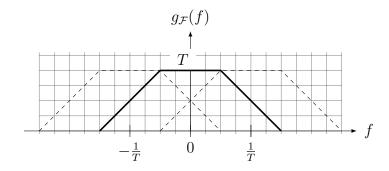
SOLUTION 2. Because  $\psi(t)$  is real, its Fourier transform is conjugate symmetric ( $\psi_{\mathcal{F}}(f) = \psi_{\mathcal{F}}^*(-f)$ ).
