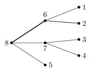
For example, in the tree shown above, nodes 1, 2, 3, 4, 5 are leaves, the probability of node 6 is given by P(1) + P(2), the probability of node 7 by P(3) + P(4), of node 8 (root) by P(1) + P(2) + P(3) + P(4) + P(5) = 1. The branch indicated by the heavy line would be labelled 6. The distance to leaf 2 is given by d(6) + d(2).
