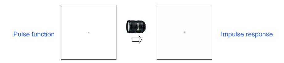
• The impulse response represents completely the optics (with a certain approximation...) and we can reproduce the same effect in image processing software
