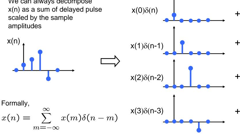
We know how to compute the output corresponding to each delayed pulse: we delay and scale the impulse response h(n) x(0)δ(n) x(0)h(n)x(1)δ(n-1) x(1)h(n-1) x(2)h(n-2) x(2)δ(n-2) x(3)δ(n-3) x(3)h(n-3) 9/11/2007 Information Sciences: Signal Processing
