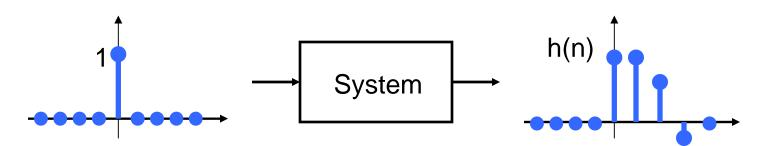
Example: impulse response of the moving average. We set g(n)=δ(n) and we compute the output y(n)=h(n). Clearly, h(n)=0, for n<0 and n>L-1 (average of L zeros) while h(n)=1/L, for n=0, ..., L-1 (average of L-1 zeros and one 1), i.e.
