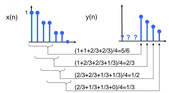
At time n the most recent samples are g(n-L+1), ...,g(n-1), g(n); therefore, the moving average is
