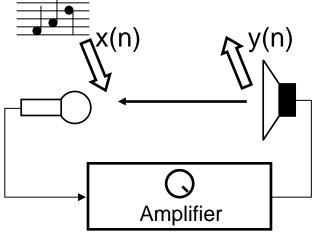
If the system has a loop gain larger than 1, any non zero input signal will trigger an unlimited output signal (theoretically...) This is called the Larsen effect
