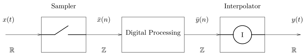
Figure 1.22: Example of a digital system that processes a continuous-time signal. The input signal is transformed to a discrete-time signal and then processed (the domain of the signals is indicated under the arrows that join the blocks). Processing includes filters and also transmission devices such as internet or disk and tape recording. The interpolator transform the result to a continuous-time signal.
