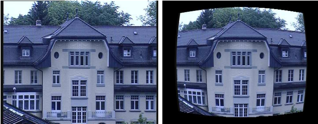
Figure 1.13: Image warping can be considered a system that transforms two-dimensional signals. On the left the original image ( 288 \times 720 pixels). On the right the output image obtained setting \rho = 2e - 6 .
