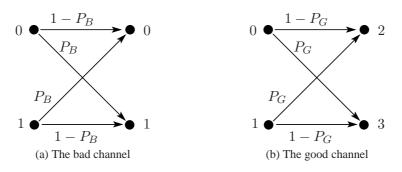
Figure 2: Two binary symmetric channels.
