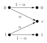
Figure 1: Binary Memoryless Erasure Channel
