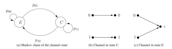
Figure 2: Binary Erasure Channel with Memory
