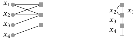
Figure 2.18: Left: Standard FG in which each variable node has degree at most 2. Right: Equivalent FSFG. The variables in the FSFG are associated with the edges in the FG.
