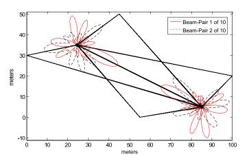
Fig. 1. Array beam-pairs associated with the two dominant singular channels of a  $10 \times 10$  MIMO channel. Beam gain-patterns are plotted on a linear scale.
