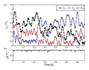
Fig. 3. (a) Magnitude of the untangled singular value sample paths of a spatially white  $3 \times 3$  MIMO channel. (b) Average singular vector correlation between adjacent samples.
