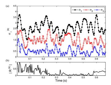
Fig. 2. (a) Singular value sample paths of a spatially white  $3 \times 3$  MIMO channel computed using strict identification conditions on singular value ordering and phase. (b) Average singular vector correlation between adjacent samples.
